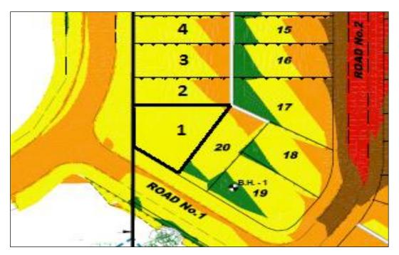
Approximate lateral extent and maximum depth of controlled filling to 1.0m. Level 1 Certification is limited to within this area.
