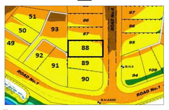
Approximate lateral extent and maximum depth of controlled filling to 1.3m. Level 1 Certification is limited to within this area.
