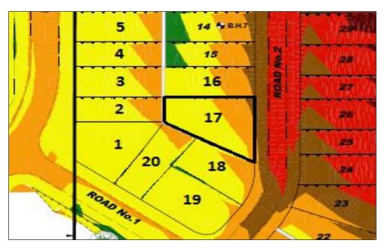
Approximate lateral extent and maximum depth of controlled filling to 1.4m. Level 1 Certification is limited to within this area.
