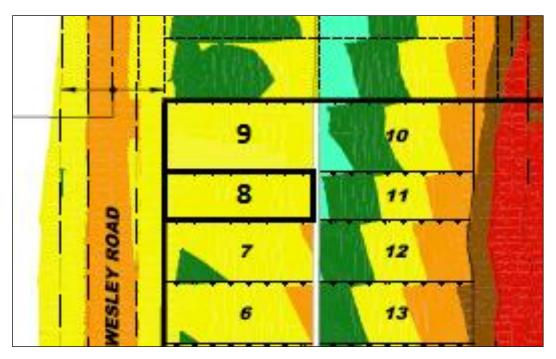
Approximate lateral extent and maximum depth of controlled filling to 1.2m. Level 1 Certification is limited to within this area.
