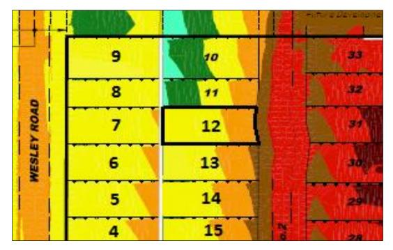
Approximate lateral extent and maximum depth of controlled filling to 1.8m. Level 1 Certification is limited to within this area.
