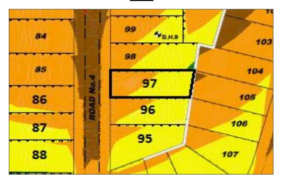
Approximate lateral extent and maximum depth of controlled filling to 0.8m. Level 1 Certification is limited to within this area.
