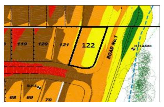
Approximate lateral extent and maximum depth of controlled filling to 0.5m. Level 1 Certification is limited to within this area.
